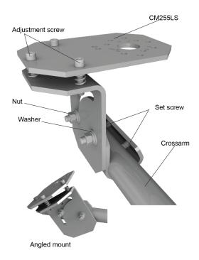
6. Verify mounting hardware is firmly tightened, and that the mounting bracket is at the desired angle. The CM255LS includes levelling bolts for additional adjustment.
