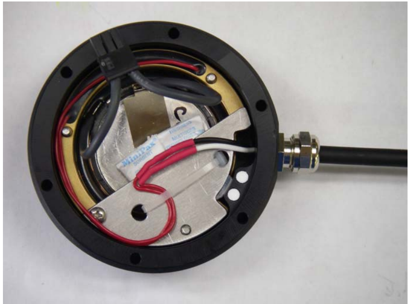
Figure 2 Complete transducer assembly with power connection
