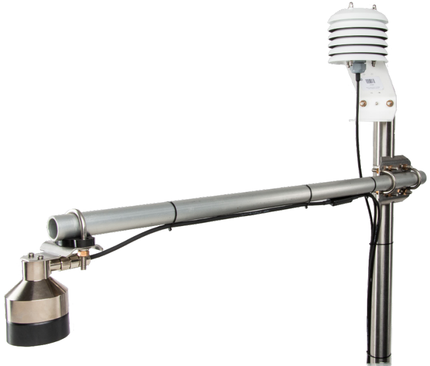
FIGURE 7-4. SR50AT-316SS Mounted to a Crossarm via the #19517 Mounting Kit with the Temperature Sensor Housed in a RAD06 Radiation Shield
