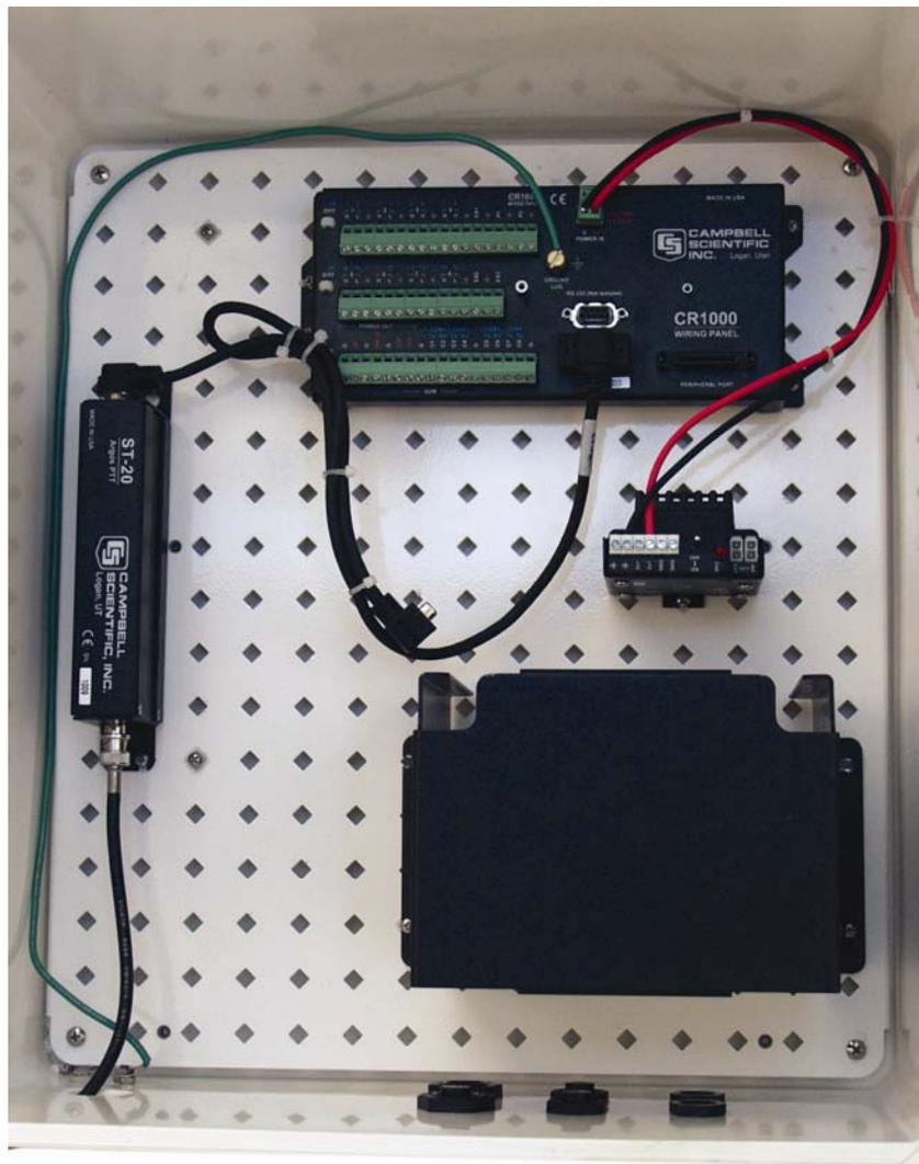
FIGURE 1-2. ST-20 with CR1000 Datalogger in Enclosure
