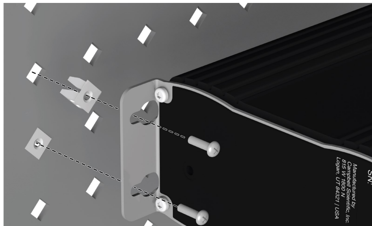
FIGURE 9-3. Enclosure backplate mounting
