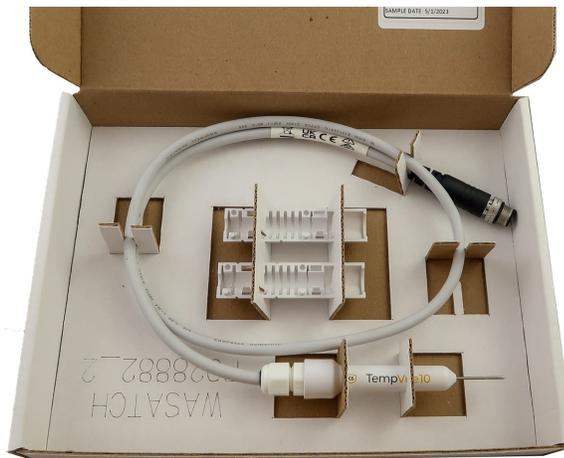
Figure 3-2. Box containing the TempVue 10 and shield extender.
