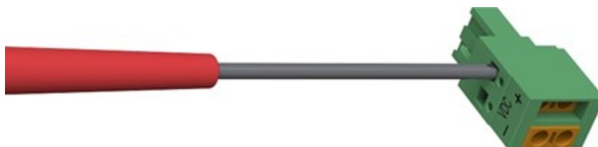
FIGURE 9-3. Opening the power connector terminals
