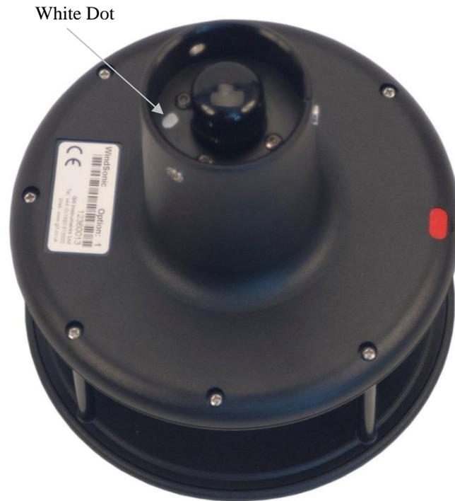
Figure 6-1. White dot indicating that the WindSonic1 has the newer settings
