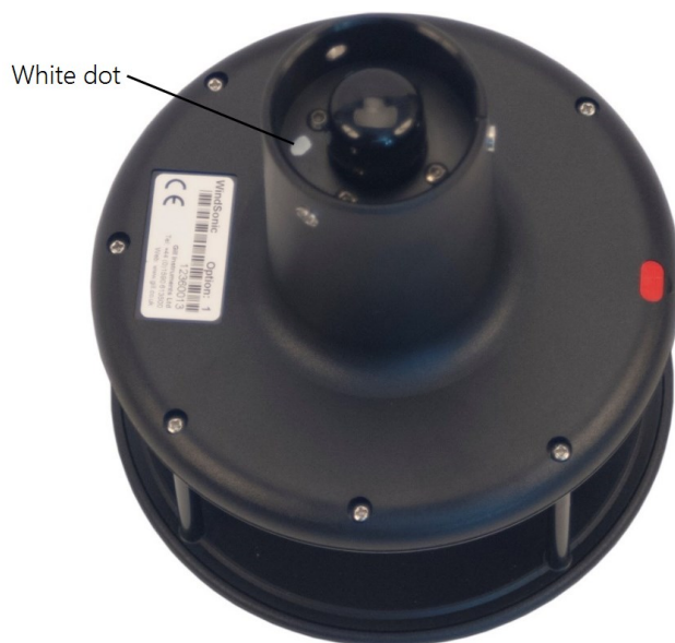
FIGURE 8-1. White dot indicating that the WindSonic1 has the newer settings
