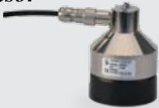
The SR50A Sonic Ranging Sensor is the smaller, better-performing upgrade of the SR50. The SR50A is made of stainless steel instead of the aluminum of the SR50. Stainless steel provides a totally conductive outer body that creates an EMF shield, resulting in more stable measurements over time. The echo processing algorithm has been improved and the size is greatly reduced.
