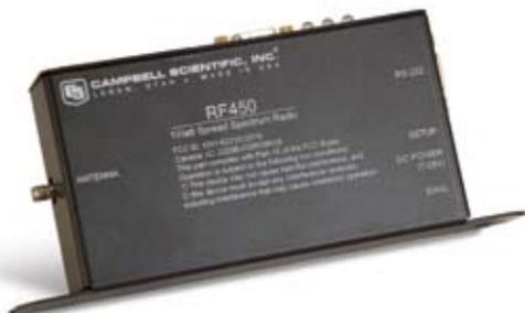
The RF450 Spread Spectrum Radio is the latest addition to our line of wireless telemetry products—transmitting over distances up to 60 miles. The RF450 is a 900-megahertz, license-free radio specifically designed to work with Campbell Scientific CRBasic dataloggers (the CR800 series, CR1000, CR3000, and CR5000). The RF450 radios consist of a radio module manufactured by FreeWave Technologies and a Campbell Scientific interface board.
