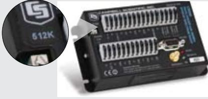
We are replacing the 1-megabit flash chip in our CR200-series dataloggers with a 4-megabit flash chip. This change increases the final storage memory from 128 to 512 kilobytes. The data format of the CR200-series is 4 bytes per data point, resulting in 128,000 data values available. Dataloggers with the 4-megabit flash chip have "512K" on their labels.
