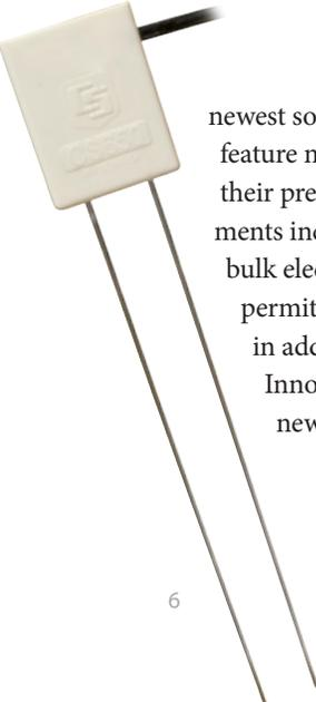
The CS650, CS655, and CWS655, our newest soil-water reflectometers, feature many improvements over their predecessors. These improvements include the ability to measure bulk electrical conductivity (EC), permittivity, and soil temperature in addition to soil-water content. Innovative techniques allow the new sensors to make accurate
