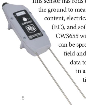
This sensor has rods that insert into the ground to measure soil-water content, electrical conductivity (EC), and soil temperature. CWS655 wireless sensors can be spread out over a field and transmit the data to a base station in a secure location away from the field.
