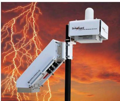
ground lightning within a 20-mi radius. To prevent false alarms, the SG000 requires an optical signal to coincide with a magnetic-field-change signal before reporting lightning.
