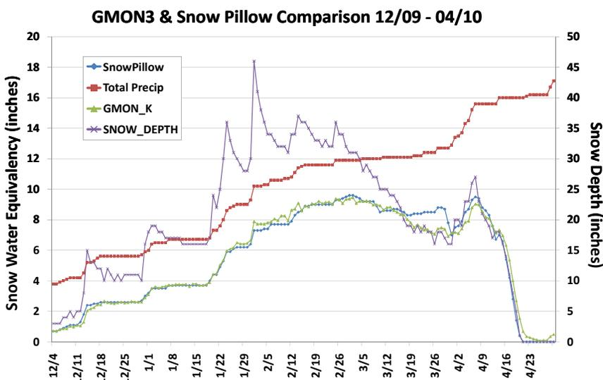
A comparison of the new GMON3 Snow Water Equivalency Sensor to a traditional snow pillow during the winter of 2009/2010 shows a strong correlation between the measurements of the two technologies.
