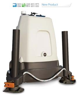
We now offer the ZephIR 300, a continuous-wave, remote sensing LiDAR system. It provides wind measurements across ten user-defined heights from 10 m to 200 m. The ZephIR 300 can be used throughout
