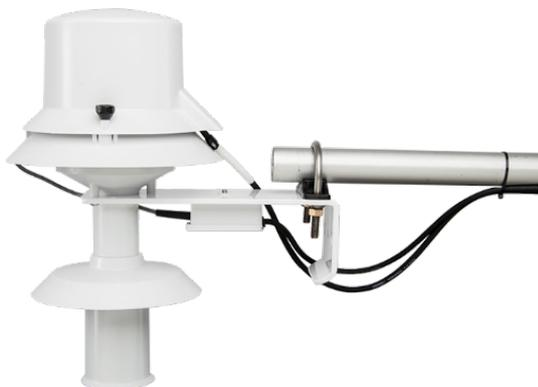
For the 2 m measurement, the 43502 attaches to the legs of a UT20 or UT30 tower via a CM202, CM203, CM204, or CM206 crossarm. Two CM210s can be used to attach the crossarm to two tower legs.
