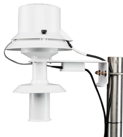
For the upper measurement, attach the 43502 to the top most mast of a UT930 tower (10 m measurement height).
