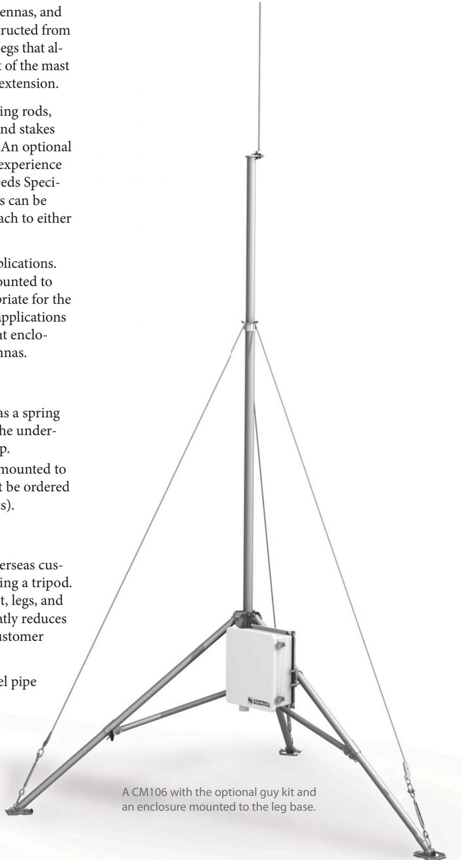
A CM106 with the optional guy kit and an enclosure mounted to the leg base.
