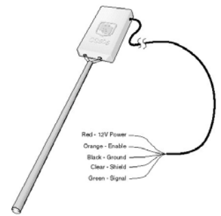
CS505 Fuel Moisture Sensor and CS505 10-hour Fuel Moisture Stick
