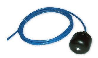
The CS512 is a rugged, low-maintenance sensor that is manufactured by OxyGuard. This sensor consists of a self-polarizing galvanic cell that generates a millivolt signal proportional to the amount of oxygen present in the measured medium (typically water). Oxygen diffuses through its membrane onto a cathode that produces a chemical reaction. An electrical current is produced by this reaction that is converted from microamps to millivolts by an inline resistor.
