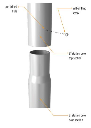
towards the West, the screw head will be located on the back side of the station.
