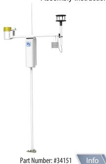
NOTE: Campbell Scientific began shipping a station pole with a new design in mid-April of 2018. Unlike the old poles which had a very tight, permanent fit, the new pole has a slip fit joint, and the pole sections must be secured together with a screw after slipping the halves together.
