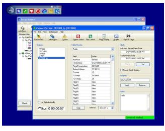
The standard Setup screen along with the Connect screen are shown above. Notes entered in the Setup screen are displayed in the Connect screen (lower right corner).
