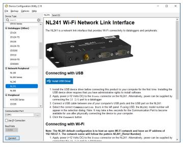
DevConfig is used to configure dataloggers, communication devices, and programmable sensors.
