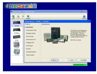
Select the EZSetup to walk through datalogger setup step-by-step.
