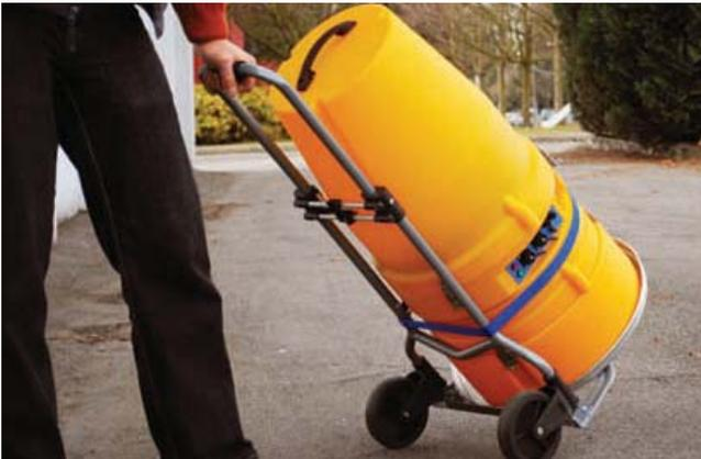
The sampler's enclosure is a molded medium-density linear polyethylene, designed to handle tough environmental challenges and weathering. Their hub has an insulated ring and a cavity for crushed ice, giving more control over the temperature of the sample.
