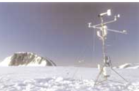
A Campbell AWS on a glacier near the Argentine Research Base, Primavera.
