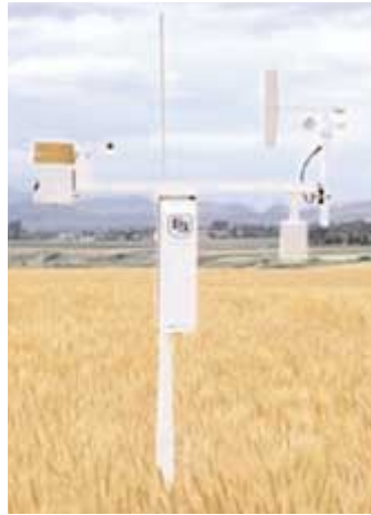
A weather station measures conditions at an Australian vineyard. Telemetry allows the grower to monitor conditions real time from their home or office.
