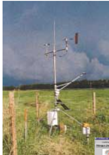
A CR10X-based weather station provides data critical to the application of pesticides as part of the North Dakota Agriculture Weather Network.
