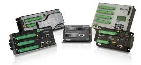
using multiplexers and other peripherals. Powerful on-board instruction sets allow unattended control decisions based on time or conditional events. For example, if measured levels are outside a predetermined range, the datalogger can sound alarms, open valves or gates, or call out to a phone to report conditions. Data are typically displayed and stored in the desired units of measure (e.g., cfs, psi, feet, inches, met**re**s, centimet**re**s).
