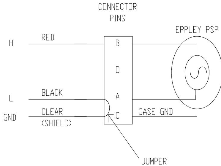
The low side of the signal is jumpered to AG to keep the signal in the datalogger's common mode range
