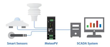
**NOTE:** The MeteoPV can be powered by USB (for configuration only), or by a 10 to 30 Vdc power supply connected to its + and - input terminals, or by power on energy (PoE). If powered by the 0 to 30 Vdc power supply or by PoE, the MeteoPV will supply 12 Vdc power to attached RS-485 sensors. The MeteoPV will not supply power to attached sensors if it is being powered only by USB.
