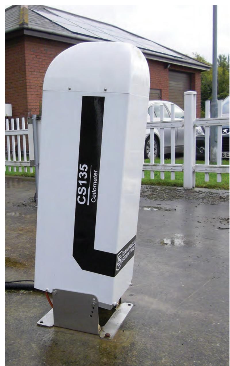
The CS135 is a ceilometer that in addition to derived cloud heights and cloud cover can also provide raw data for an end user to interpret as they wish. Various detection parameters are configurable but the end user can always be clear exactly how 'raw' data has been pre-processed.
