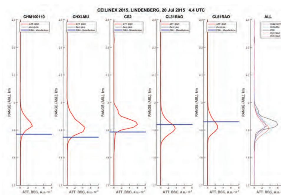
Different ceilometers may agree well in producing a scatter profile but clearly use very different algorithms in calculating the cloud height. The graphs show data from the 2015 'Ceilinex' campaign and are produced courtesy of Frank Wagner, DWD.
