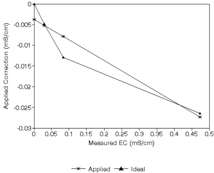
**FIGURE 8.1-1. Plot of Ideal and Actual Correction between 0 and 0.44 mS cm<sup>-1</sup>**
