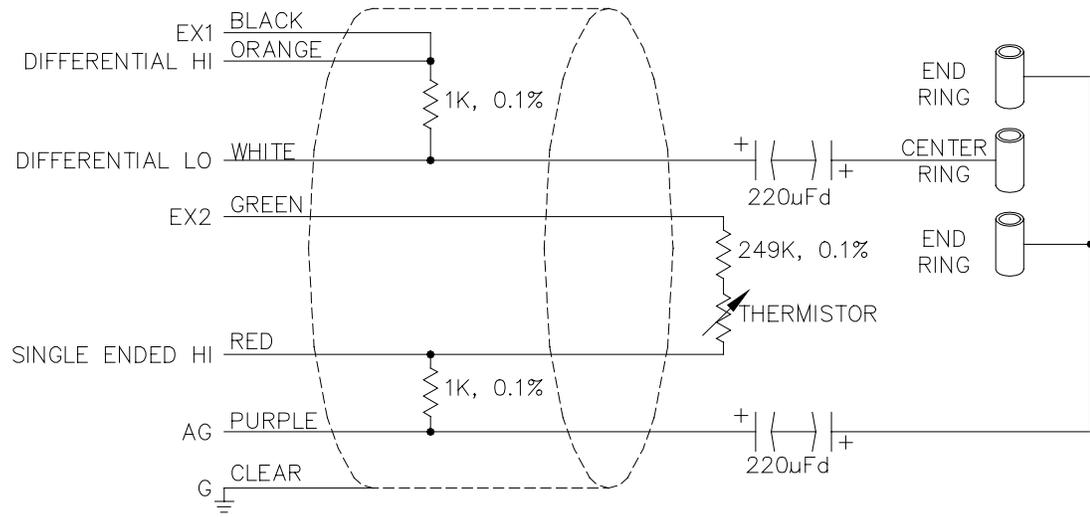
FIGURE 11-1. 247 Conductivity and Temperature Circuit Diagram
