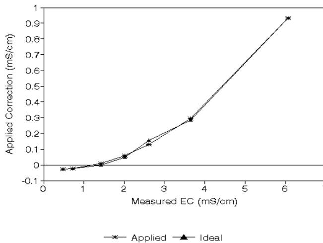
**FIGURE 8.1-2. Plot of Ideal and Actual Correction between 0.44 and 7.0 mS cm<sup>-1</sup>**
