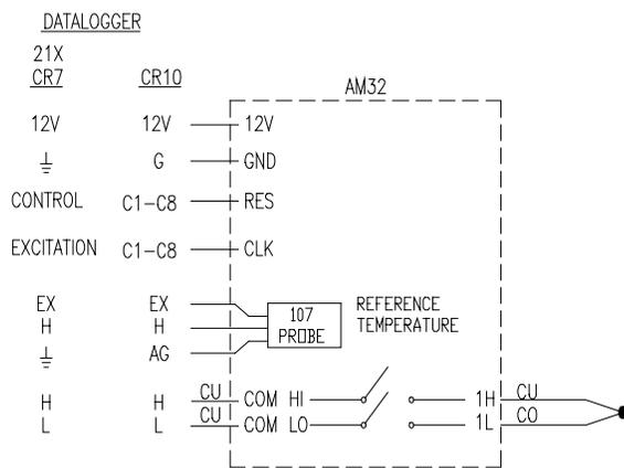
**FIGURE 6-2. Differential thermocouple measurement with reference junction at the AM32.**
