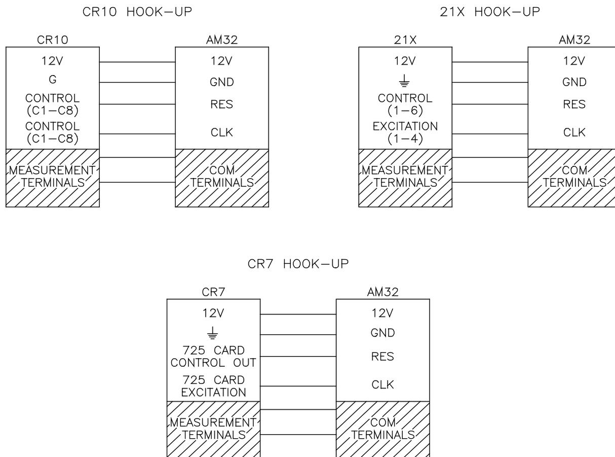
FIGURE 3-1. Hook-up diagrams for datalogger to AM32 connections.
