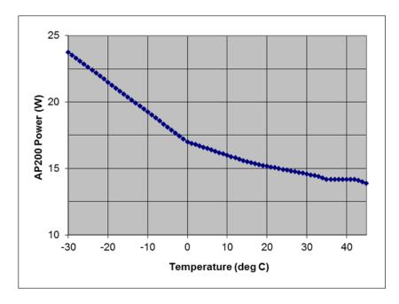
FIGURE 4-23. Average power consumption relative to temperature
