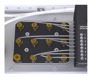
FIGURE 5-6. Labelled inlet connections inside enclosure
