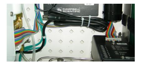
FIGURE G-2. Bundled cable of power adapter
