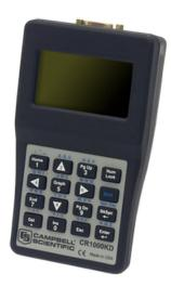
FIGURE 4-11. CR1000KD handheld keyboard/display
