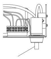
FIGURE 7-3. Correct reassembly after filter replacement
