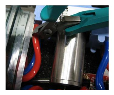
FIGURE J-9. Location of cuts to remove pump assembly from tubing
