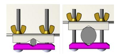
FIGURE 5-2. Mounting clip orientation for pipe diameters between 1.3 and 3.8 cm
