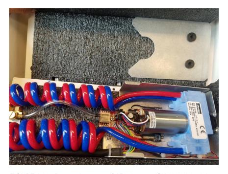
FIGURE J-12. Proper placement of AP200 pump (SN 33240) back into foam of pump enclosure.
