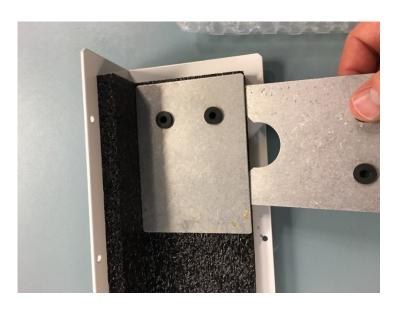
FIGURE J-4. Removal of original pump module inner plate and replacement with new inner plate provided in pump replacement kit (pn #33241)
