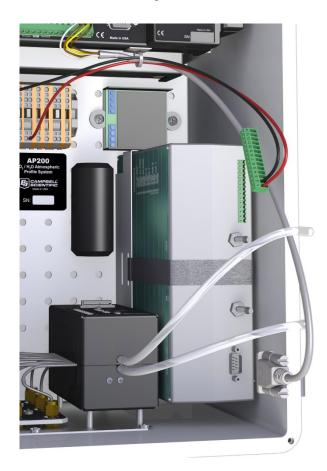
FIGURE 7-5. Components and fittings of IRGA installation
