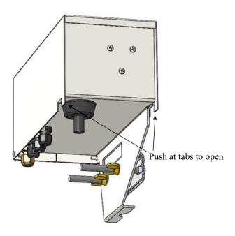
FIGURE 5-14. Tabs for opening intake assembly
