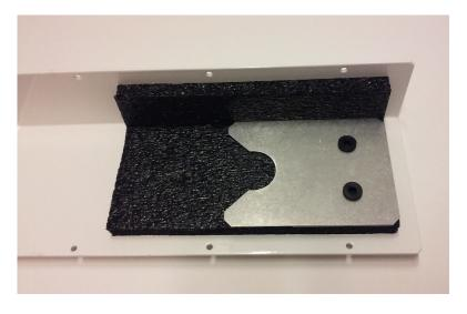
FIGURE J-6. New inner plate placement on pump module cover
