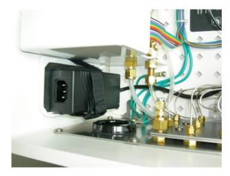
FIGURE 4-8. AC/DC power adapter kit installed in AP200
