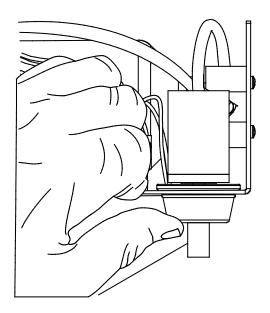
FIGURE 7-1. Releasing rain diverter from intake assembly
