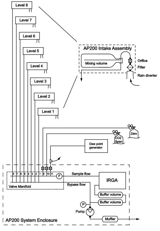
FIGURE 4-17. Plumbing diagram of AP200 system
