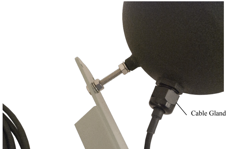
FIGURE 6-3. BlackGlobe fitting and cable alignment
