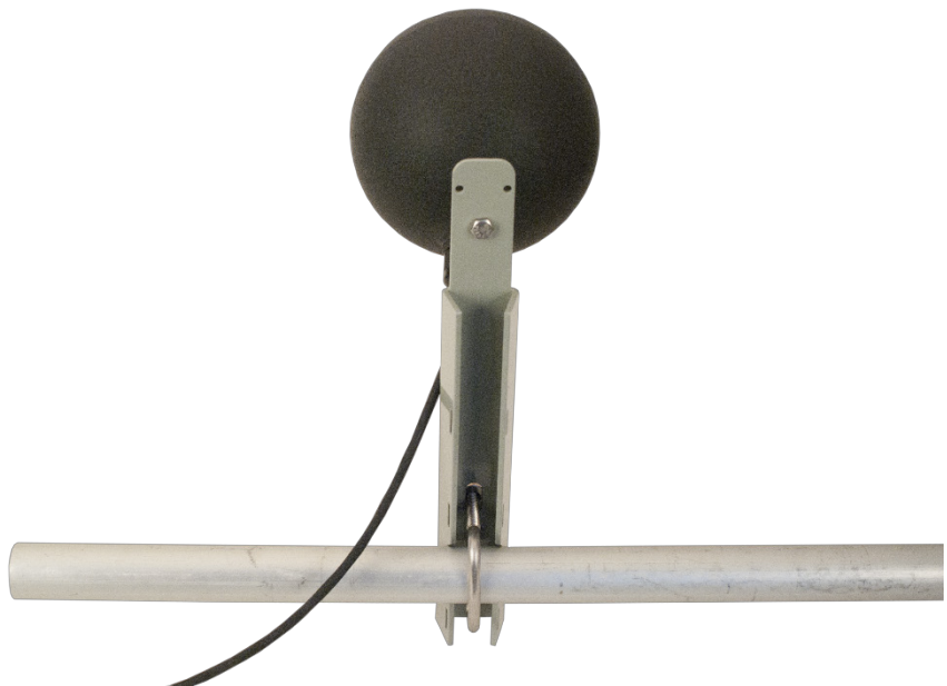
FIGURE 6-5. BlackGlobe mounted to a crossarm (back view)
