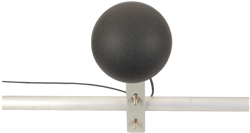
FIGURE 6-4. BlackGlobe mounted to a crossarm (front view)
