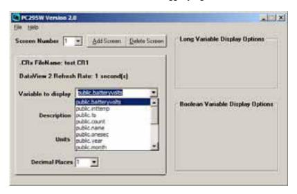
6. The 'Description' and 'Units' fields are free-form text strings that are displayed on the CD295 along with the value collected from the datalogger. These fields can be used to provide a user friendly description and engineering units of the value displayed. It is also possible to choose the number of decimal places to be used when displaying the value.
