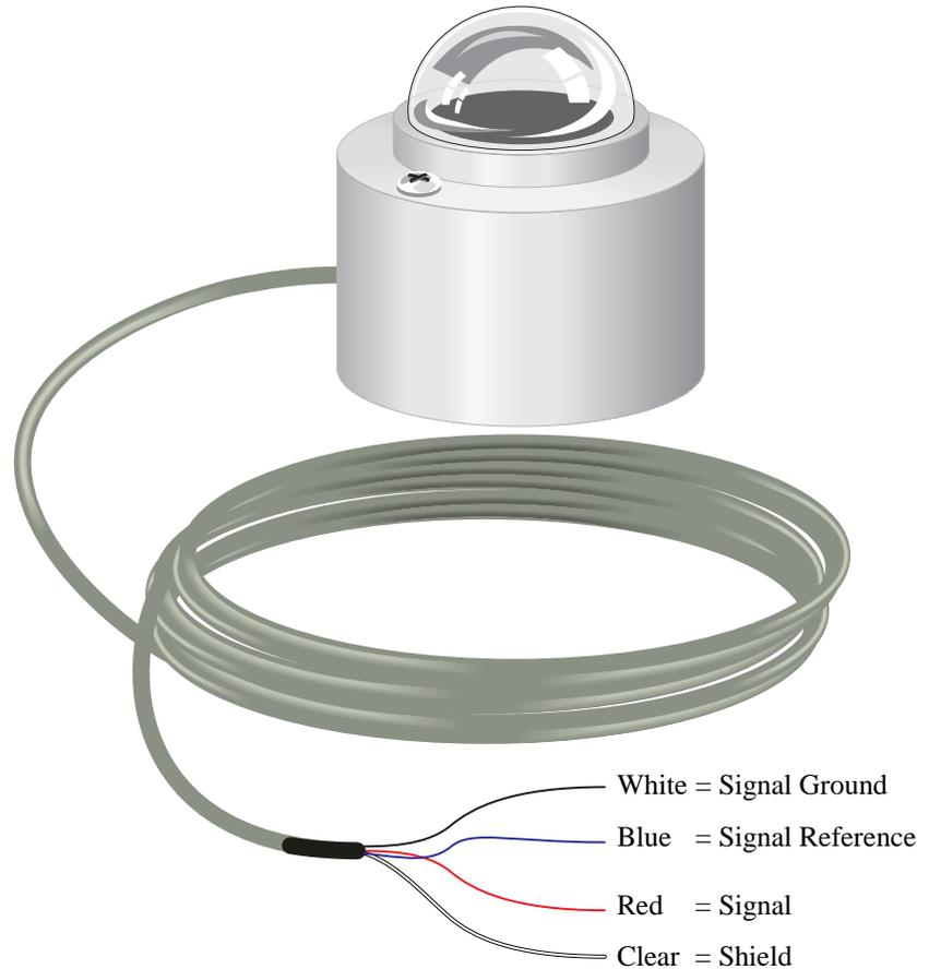
FIGURE 4-1. CM3 Wiring
