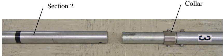
FIGURE 2.2-7. Mast Section 2 and Mast Section 3
