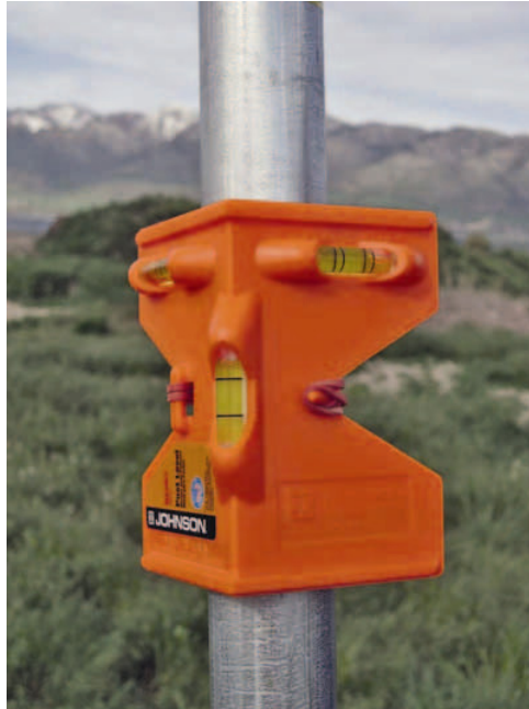
FIGURE 2.5-2. Pole Level Ensures Vertical Mast
