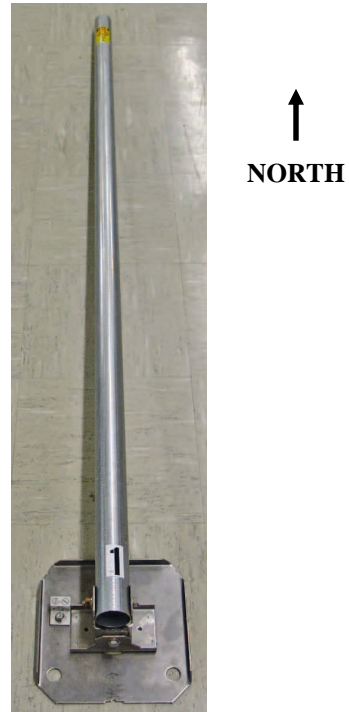
FIGURE 2.2-3. Mast Section 1 Oriented on Base
