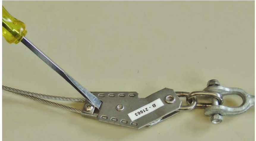
FIGURE 2.4-9. Adjusting Cable through Wedge Clamp
