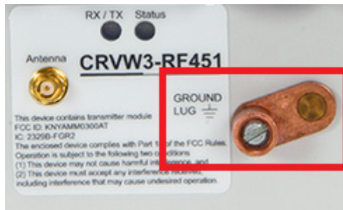
FIGURE 8-15. CRVW3 Ground Lug Location
