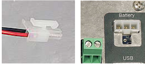
FIGURE 8-8. –ALK Battery Pack Connector Cable and CRVW3 Battery Connection
