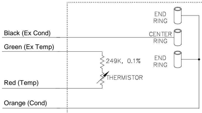
FIGURE 13-1. CS547 Conductivity and Temperature Circuit Diagram
