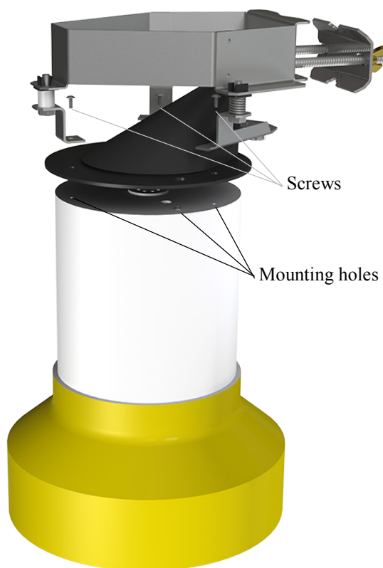
FIGURE 6-6. Mounting CM270 to the rain gauge
