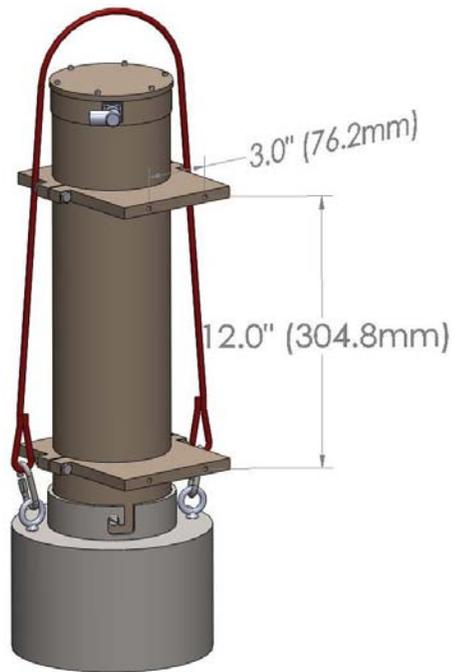
Figure 9-1. Position of 1/4 - 20 mounting holes
