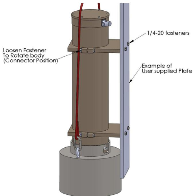
Figure 9-2. Example of wall/plate mounting
