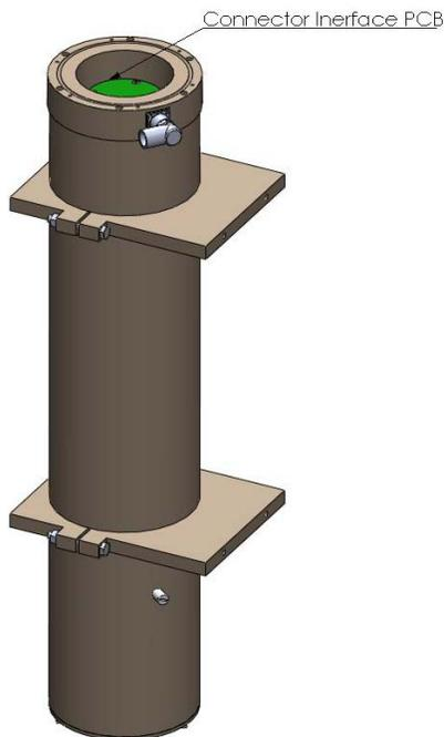
Figure 14-4. CS725 with top cap removed
