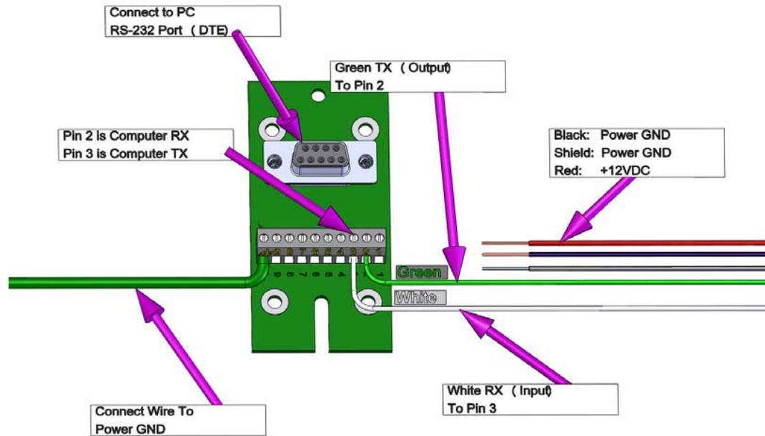
Figure 4-1. CS725 connection to DB9F-TERM
