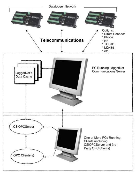
The diagram below depicts the flow of information between the datalogger network, LoggerNet communications server, LoggerNet client applications, and remote clients.
