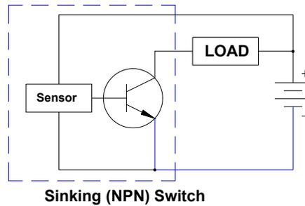
The **Sinking** method connects or switches one side of the load to the negative (-) side of the power supply. The positive (+) side is connected directly to the other side of the load as shown. “**NPN**” refers to the type of transistor used to act as a switch in this type of solid-state sensor.
