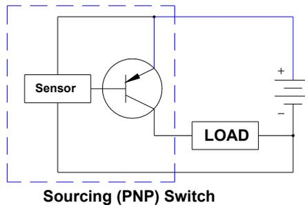
The **Sourcing** method connects or switches one side of the load to the positive (+) side of the power supply. The negative (-) side is connected directly to the other side of the load as shown. “**PNP**” refers to the type of transistor used to act as a switch in this type of solid-state sensor.
