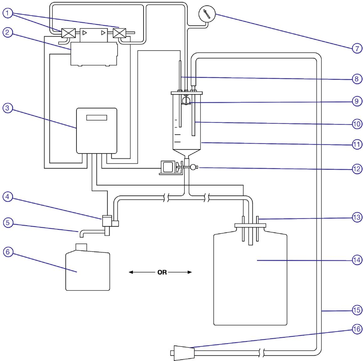
FIGURE 1-3. Diagram of the CVS/BVS Vacuum System
