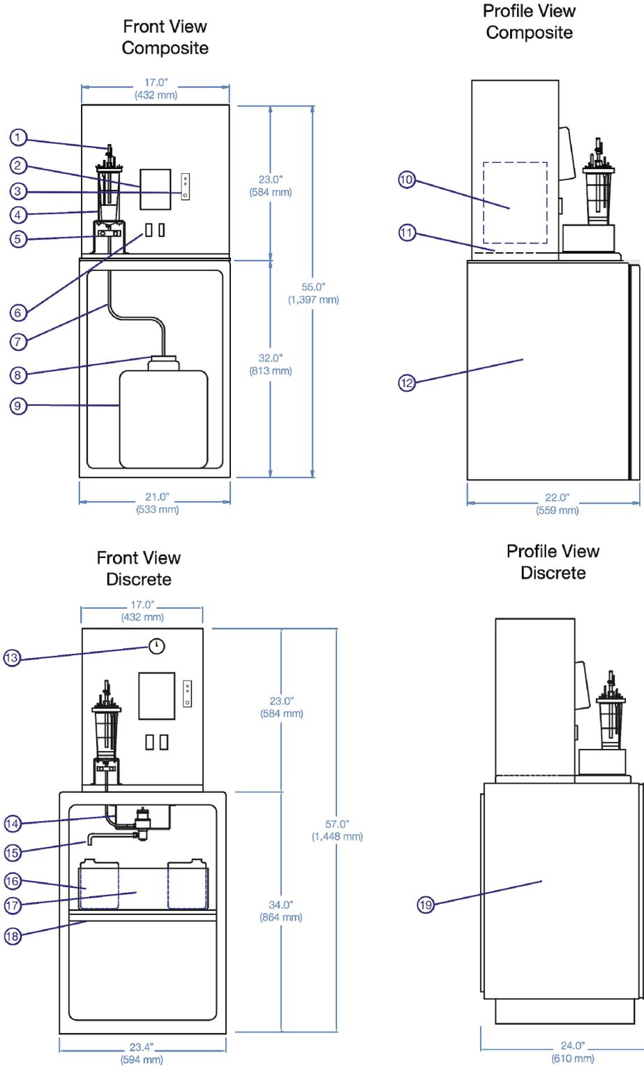
FIGURE 1-2. Diagrams of the CVS4200 Basic Unit
