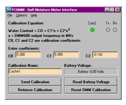
FIGURE 4. PCDMM User Interface Display
