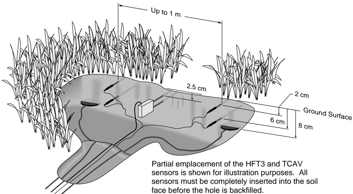
**FIGURE 2.5-1. Placement of Thermocouples and Heat Flux Plates**
