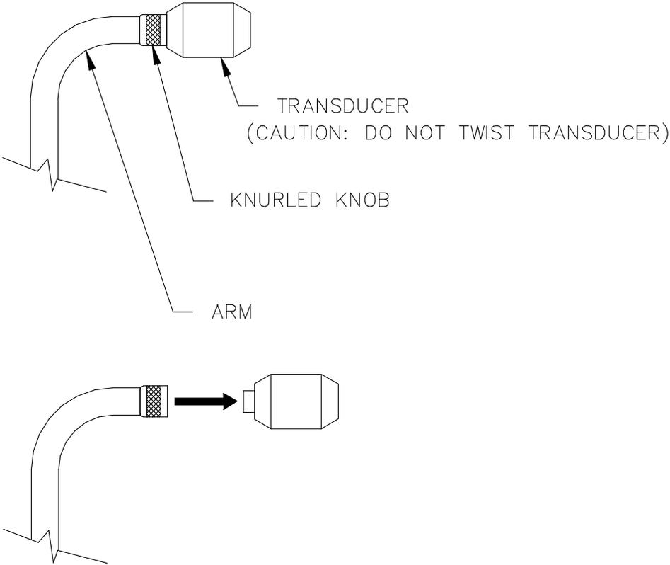
**FIGURE B-1. CA27 Transducer and Arm**
