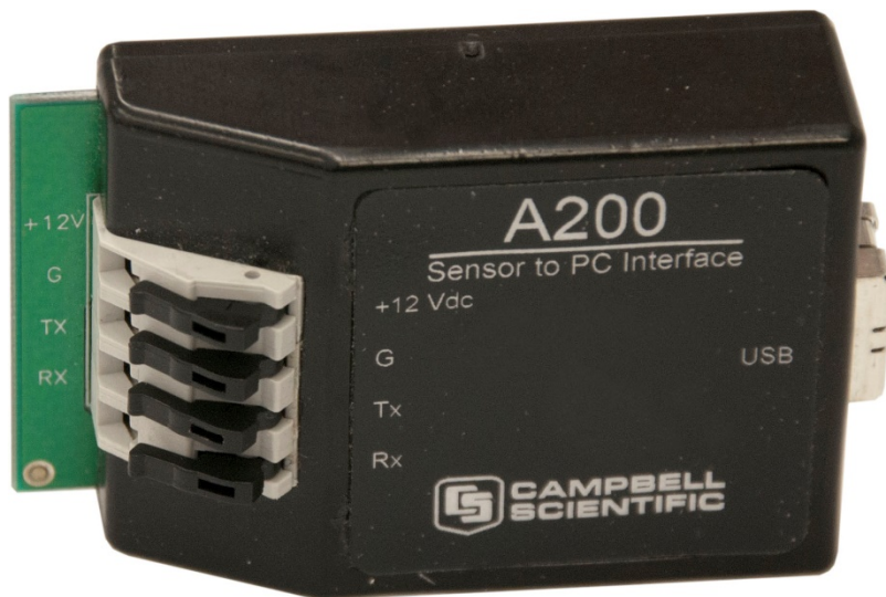
FIGURE A-1. A200 Sensor-to-PC Interface
