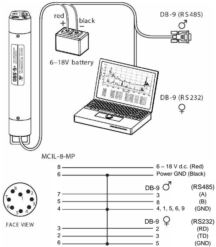
Figure 6-1. Electrical connections
