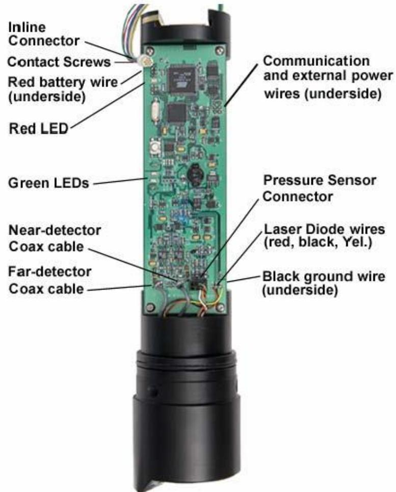
Figure 8-1. Internal components
