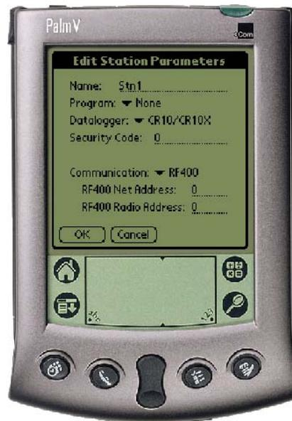
When you are finished editing the station parameters, touch **OK**. You will be returned to the *Stations* window. PConnect has three main windows: the *Stations* window, the *Files* window, and the *PConnect Settings* window. You can navigate between the windows by pressing the window's name in the upper right corner of the screen.
