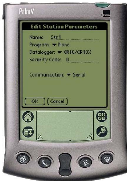
From this window you can change the station **Name**, associate a **Program**, change the **Datalogger** model, enter a **Security Code**, and select the mode of **Communication**.
