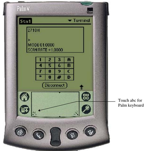
For all dataloggers except the CR1000, CR200(X), CR800/850, and CR3000, the datalogger's keyboard/display keypad is depicted on the *Terminal* window. The Palm device's graffiti pad or keyboard can also be used to enter characters. For CR1000, CR800/850, CR200(X), and CR3000 dataloggers, there is no keyboard/display depicted, so the graffiti pad or keyboard must be used.
