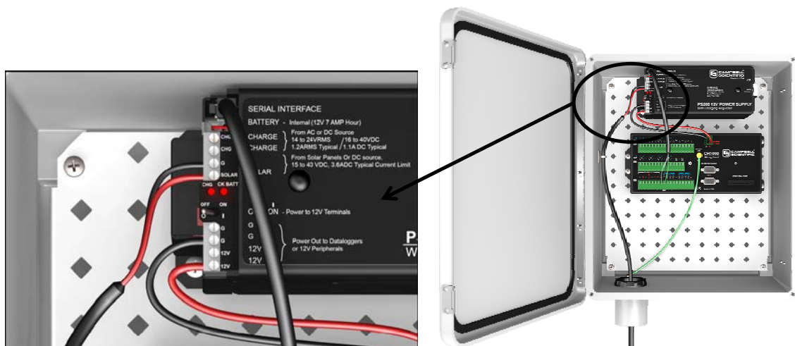
Figure 2-2. The PS200 connected to a CR1000 and solar panel.
