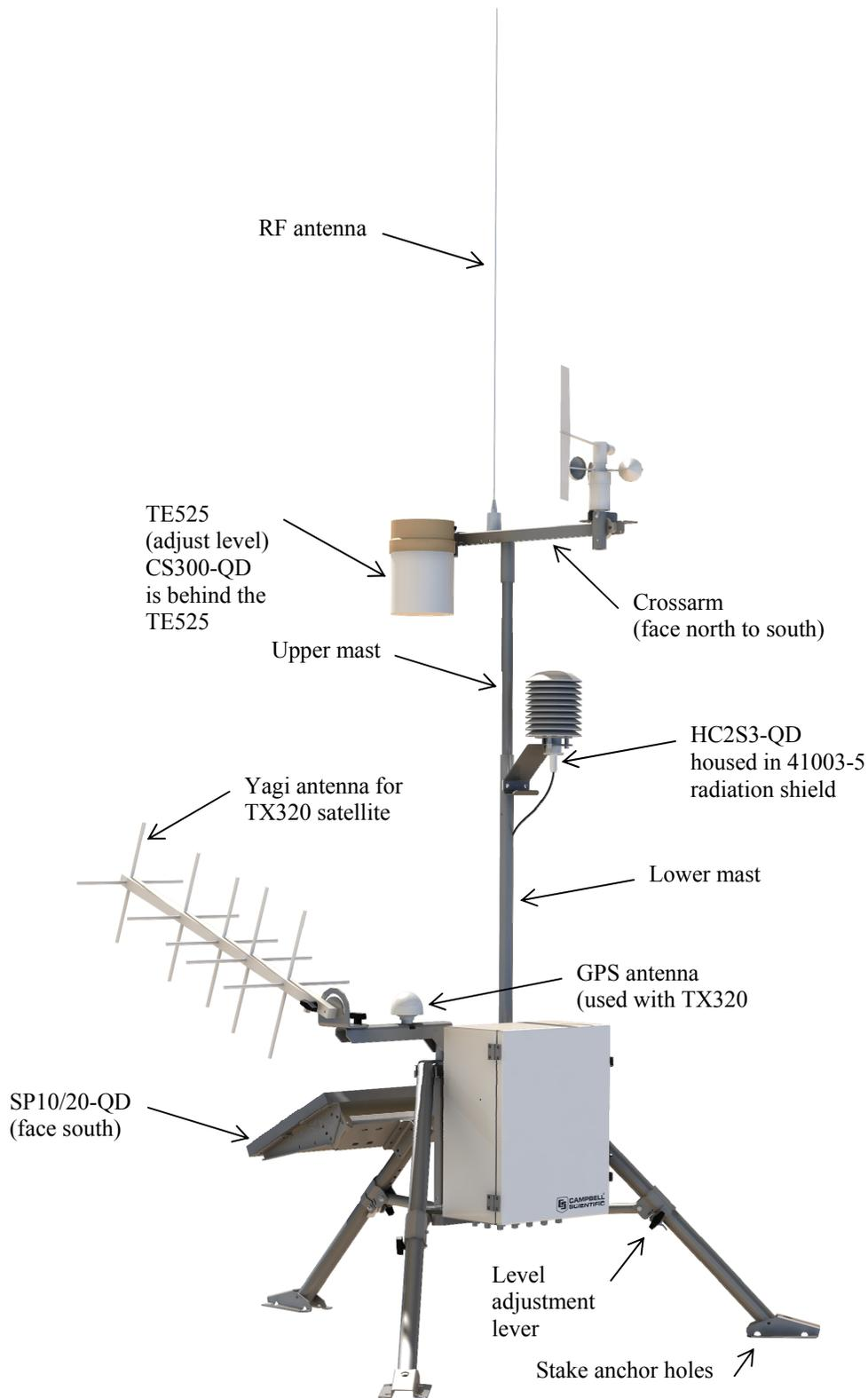
FIGURE 1-2. RAWS-F Quick Deployment Weather Station. Some wiring not shown.
