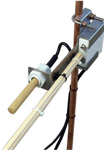
FIGURE 4.7-1. CS516-QD Fuel Moisture/Fuel Temperature
