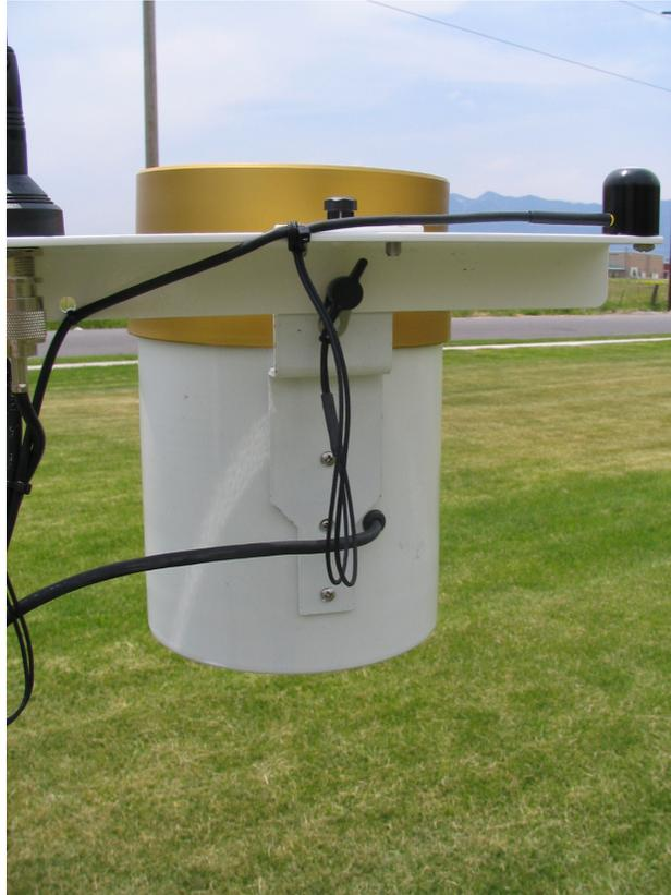
FIGURE 4.3-1. Rain gage and CS300-QD pyranometer
