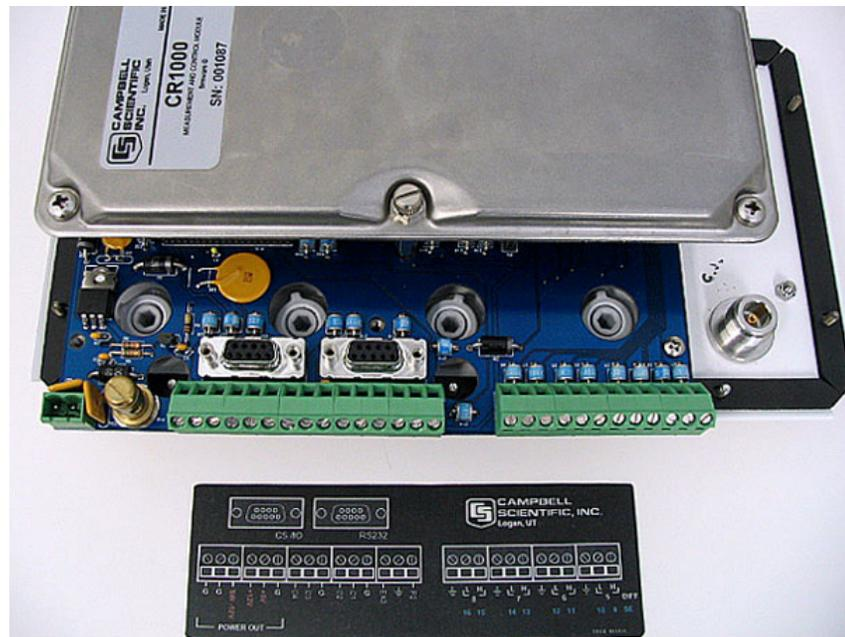
FIGURE 5.7-1. CR1000 and printed circuit wiring panel
