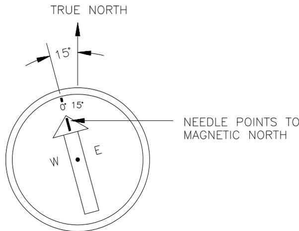
FIGURE 7.3-3. A declination angle west of True North (negative) is subtracted from 0 (360) degrees to find True North
