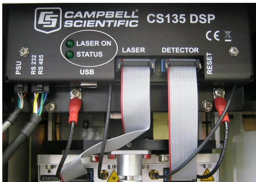
FIGURE 7-3. Diagnostic LED indicators
