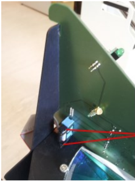
Levers to help remove ribbon connector
