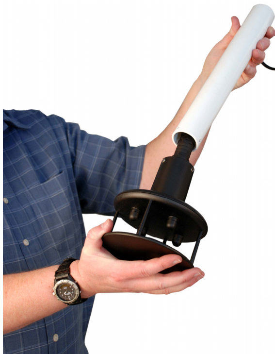
FIGURE 2.4-10. Gill WindSonic Connected to Cable
