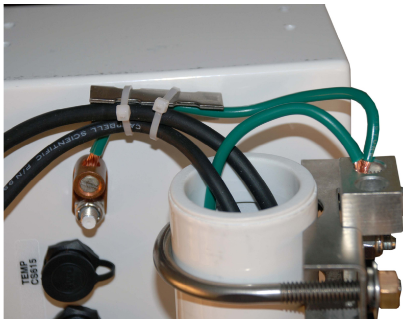
FIGURE 2.6-2. Grounding to Lightning Rod Clamp
