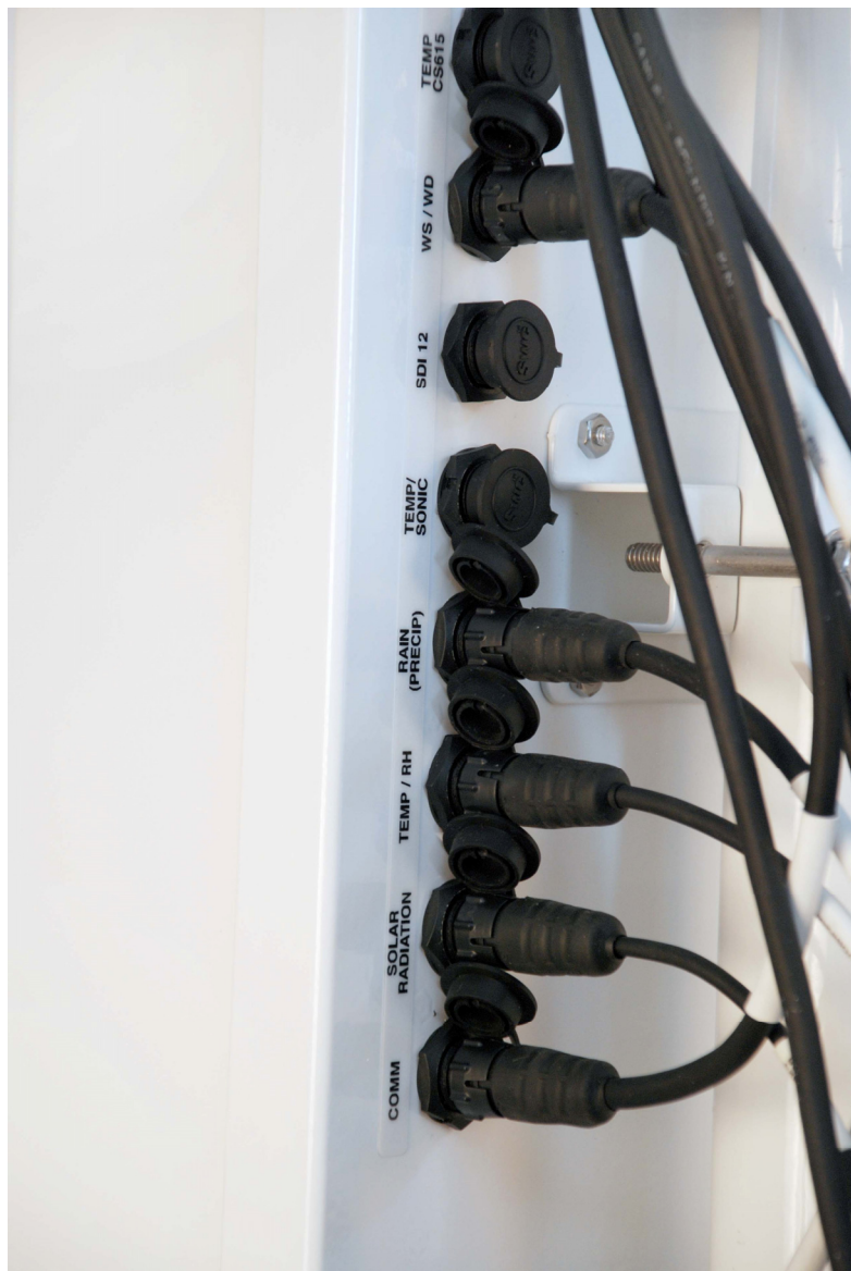
FIGURE 2.4-15. Connecting Sensor Cabling to Enclosure
