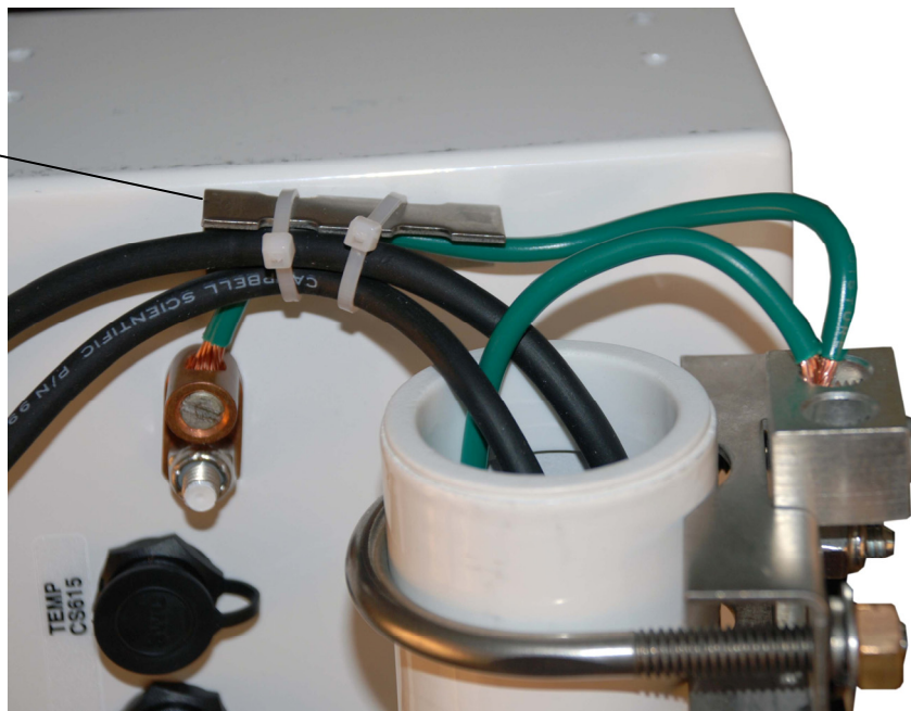
FIGURE 2.9-1. Cabling Strapped to Wire Tie Harness
