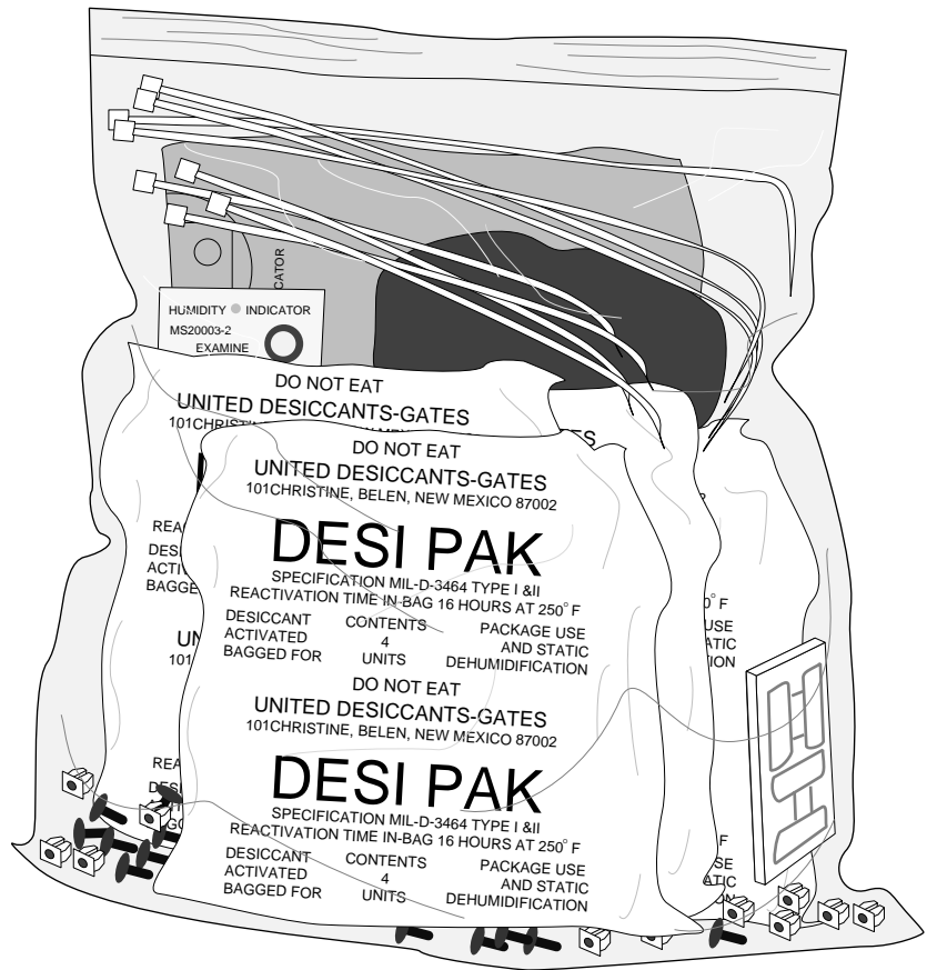
FIGURE B.1-3. Enclosure Supply Kit
