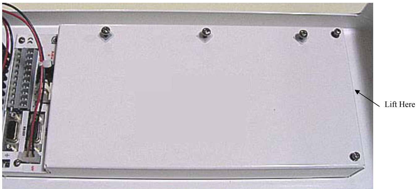
FIGURE 2.4-7. Removal of the Electronics Cover
