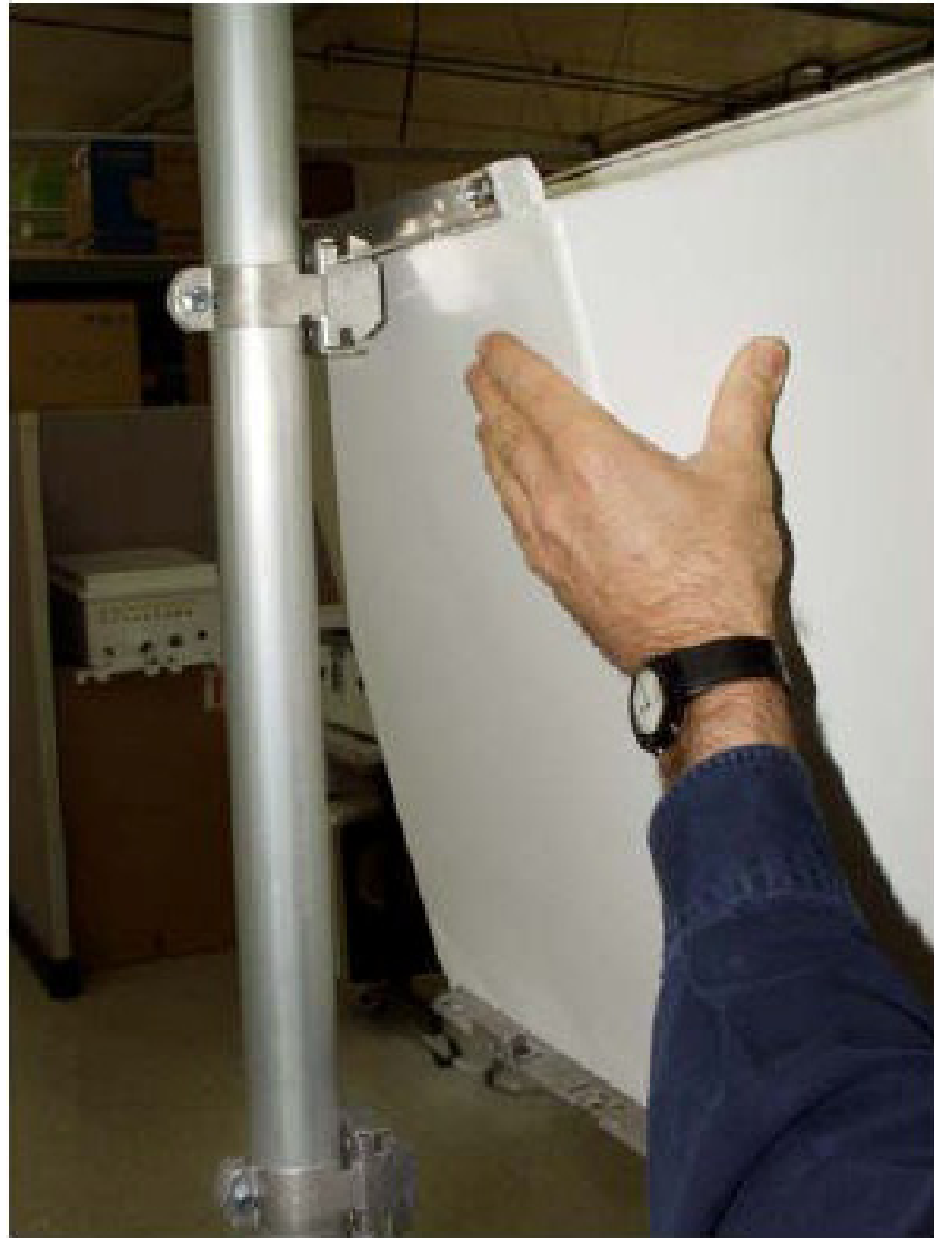
FIGURE B.2-3. Top Clamp Hook Side Up
