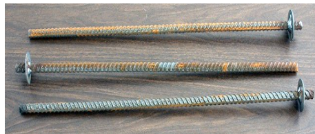
FIGURE 2-6. For temporary sites, drive the stakes of the 16773 Tripod Stake Kit (left) through the center hole in each tripod foot (right). The stakes should be driven in until they barely contact the foot surface. For permanent sites, install user-supplied bolts through the holes in each tripod foot.
