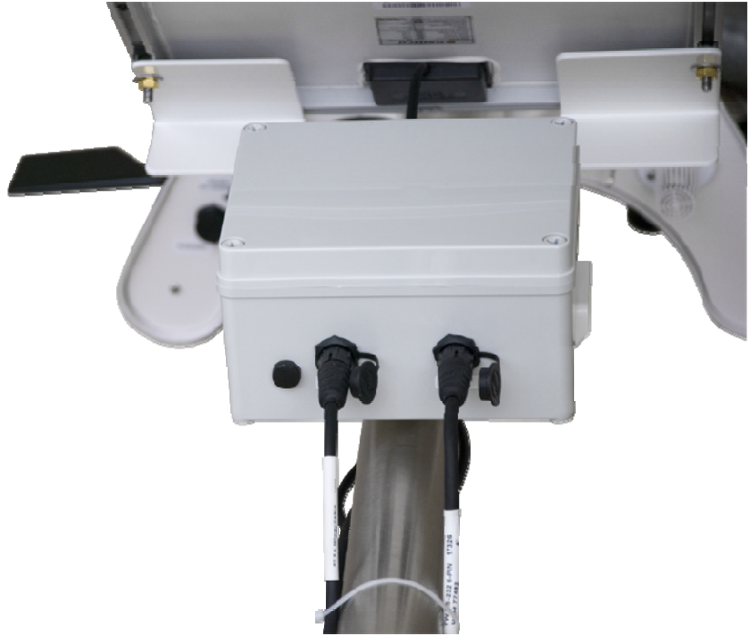
FIGURE 2-17. The Cables Connected to Enclosure
