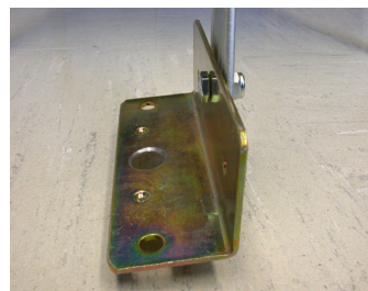
FIGURE 2-6. For temporary sites, drive the stakes of the 16773 Tripod Stake Kit (left) through the center hole in each tripod foot (right). The stakes should be driven in until they barely contact the foot surface. For permanent sites, install user-supplied bolts through the holes in each tripod foot.
