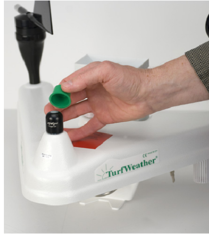
FIGURE 2-11. The red or green cap protects the solar radiation sensor while the weather station is being shipped and installed. Accurate measurements require the cap to be removed
