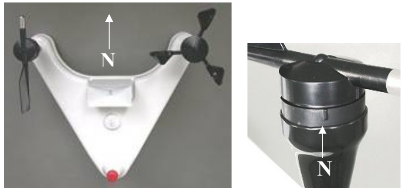
FIGURE 2-9. Accurate wind direction measurements require the reference line on the wind direction sensor (right) to be aligned with Magnetic North.
