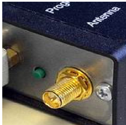
FIGURE 1-5. The connector marked Antenna on an RF401-series radio is where the antennas attach.
