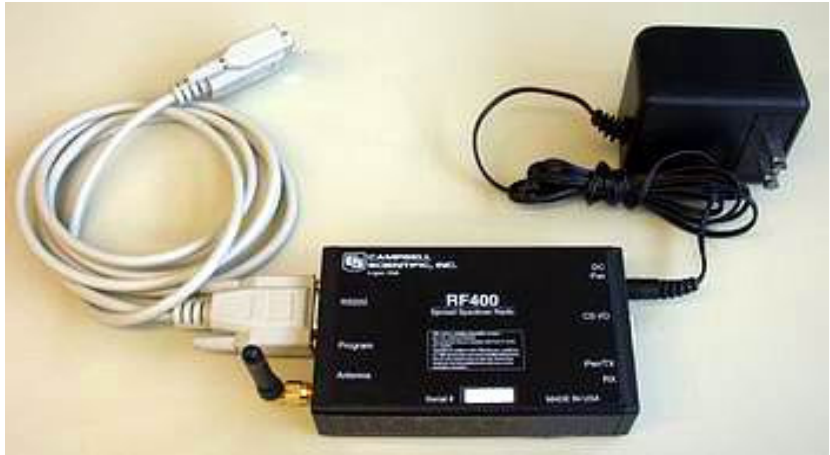
FIGURE 1-6. Radio connections. The serial cable (left) connects to the port marked RS232 and the AC adapter connects to the port marked DC Pwr input.
