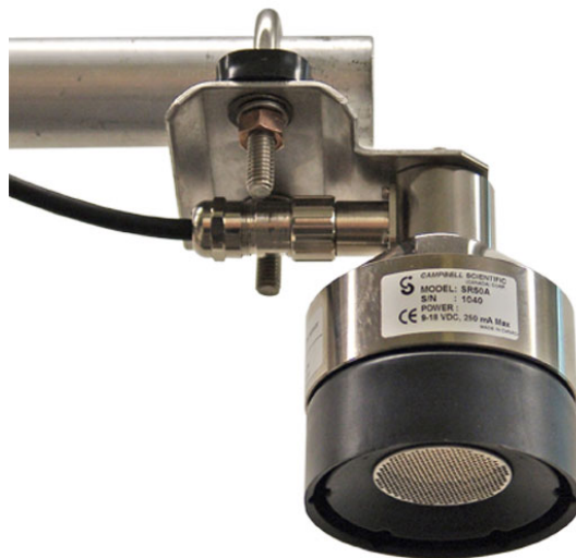
FIGURE 4.12-4. The SR50A Mounted to the Crossarm Shown from Another Angle
