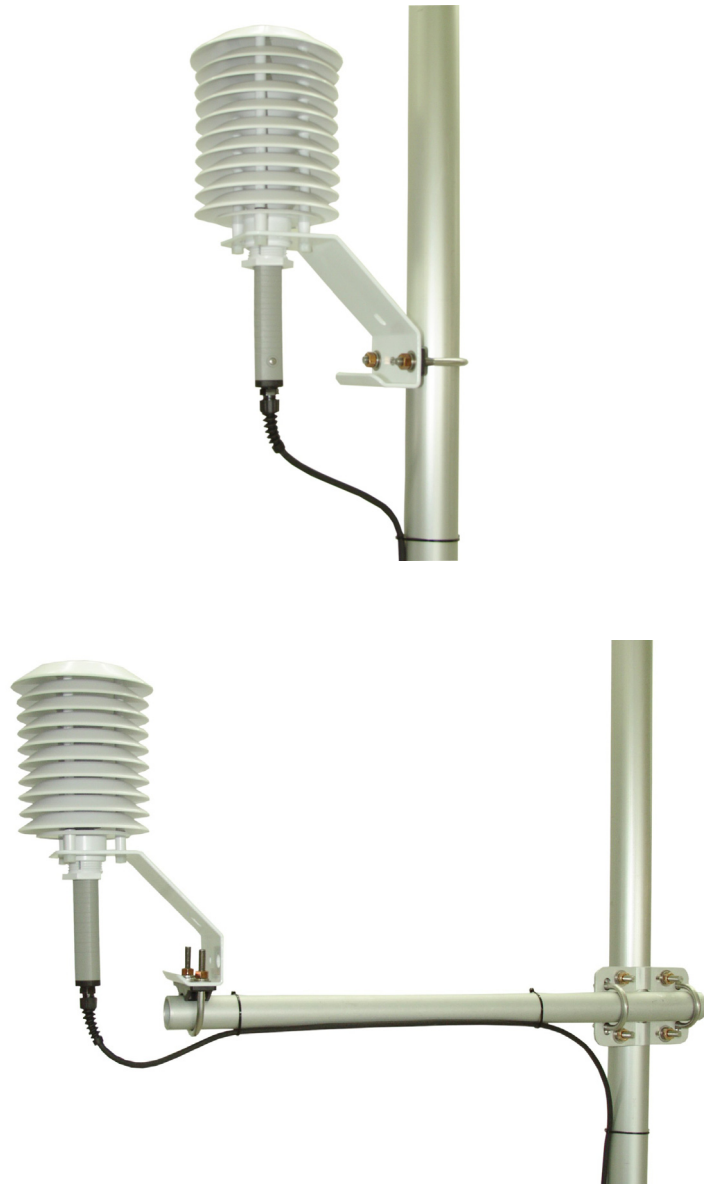
FIGURE 4.8-1. HMP45C Vaisala Temperature and RH Probe
