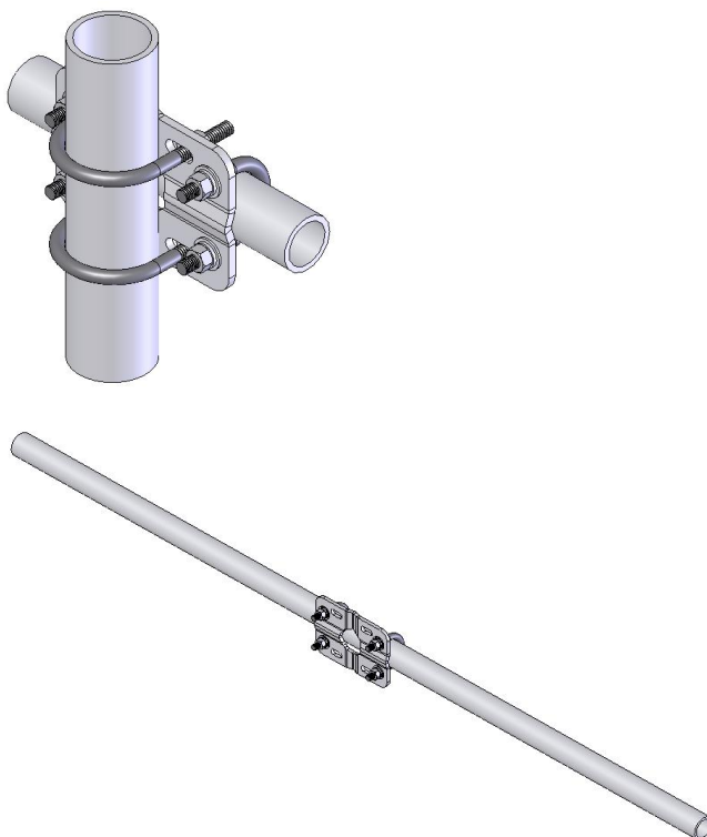
FIGURE 2.2-2. CM210 crossarm-to-pole bracket (top) is included with the crossarm for attaching the crossarm to the tower's mast or leg
