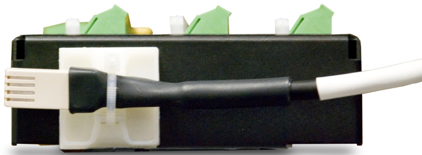
FIGURE 4.16-1. CS210 installed on a CR1000
